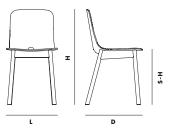
DIMENSIONS L 450 x D 510 x H 780 mm L 17.7 x D 20 x H 30.8 "
