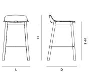
DIMENSIONS L 422 x D 428 x H 776 mm L 16.6 x D 16.8 x H 30.5 "
